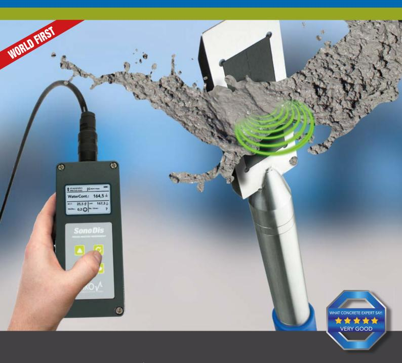
Based on state-of-the-art TRIME® radar technology it is possible for the first time ever to measure and analyse the water content, quickly, precise and direct on site.
